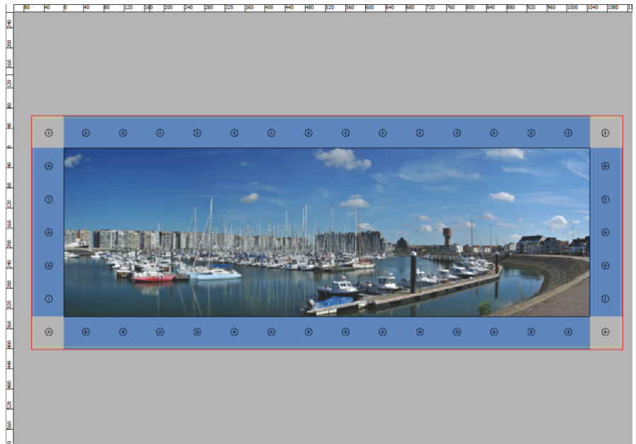
Figure 4.22: Grommets (circles with cross) in the extensions
