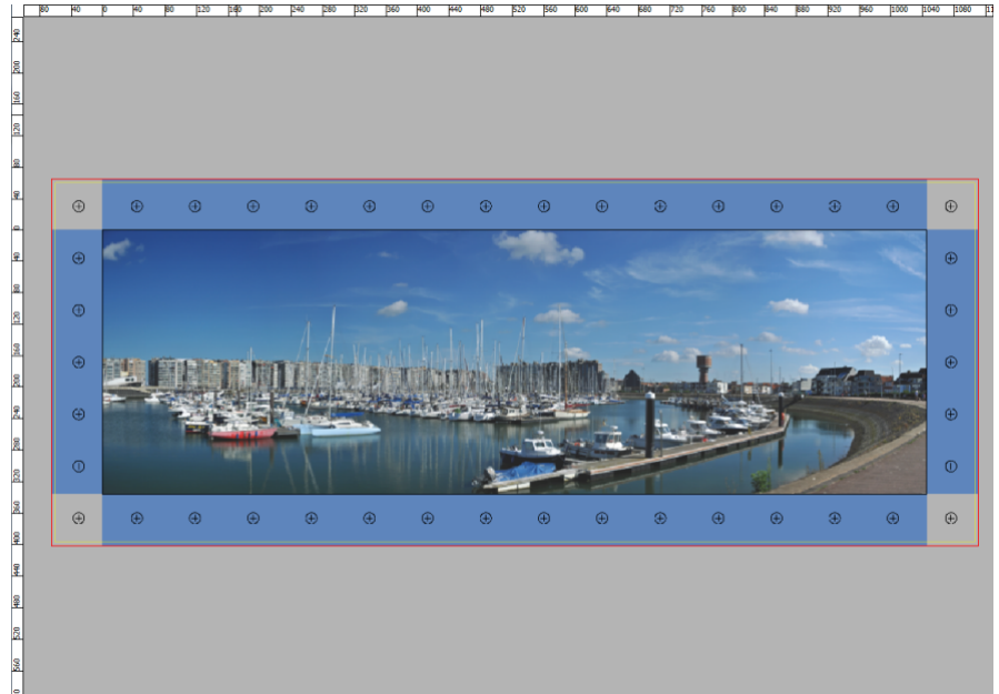
Figure 4.22: Grommets (circles with cross) in the extensions
