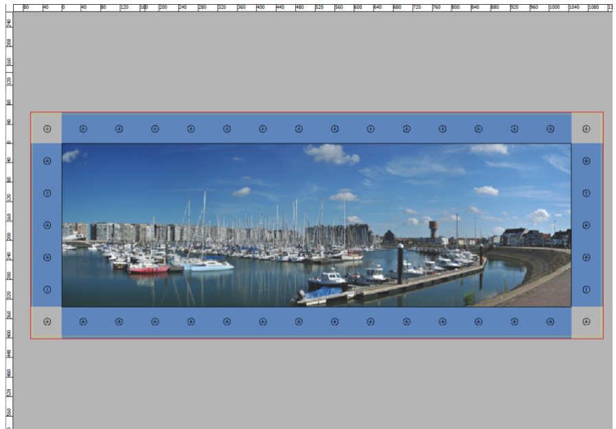
Figure 4.22: Grommets (circles with cross) in the extensions
