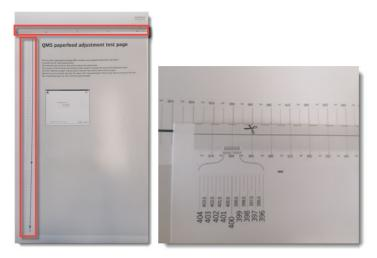
The lengths of the two rulers should match. Cut the horizontal one and position it precisely next to the vertical one. Make sure that the zero points are placed on top of the other. Look for a significant distance (400 mm), and check the distance from the horizontal guideline. In this example, the reference value is 400,00 mm with a measured length of 400,50 mm.
